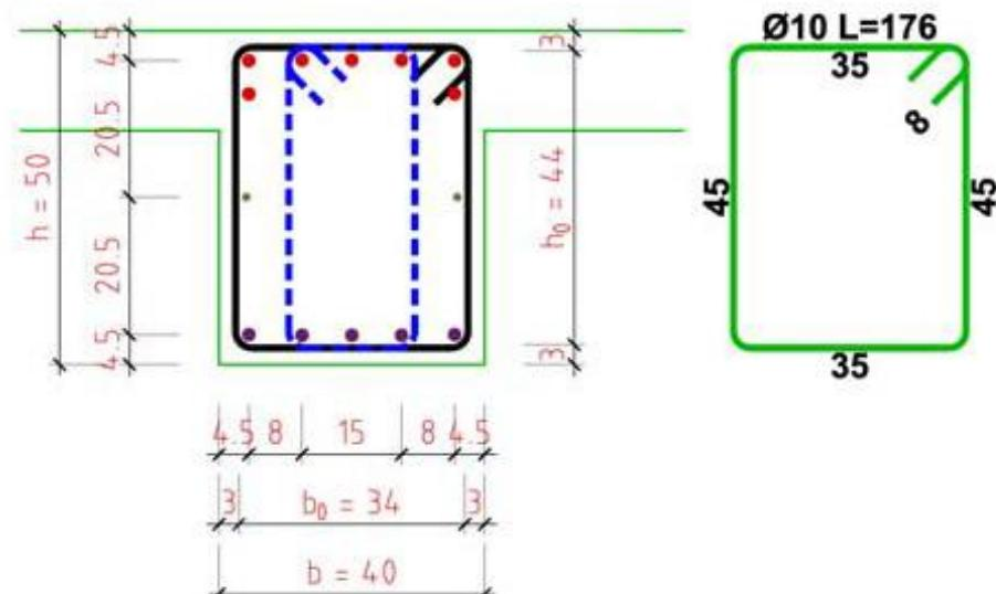
$$\frac{m \times a_{sw}^{(1)}}{s} = \frac{341.6}{38.7 \times 43.5 \times \cot 45^\circ} = 0.203 \frac{\text{cm}^2}{\text{m}}$$
