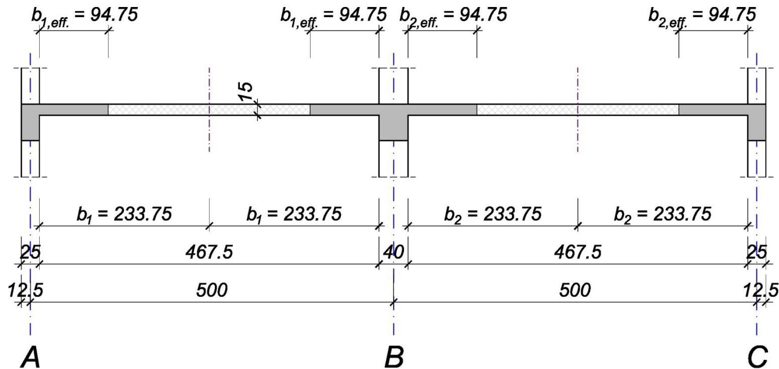
$$b_{1,\text{eff.}} = b_{2,\text{eff.}} = 0.2b_1 + 0.1L_0 \leq 0.2L_0$$
