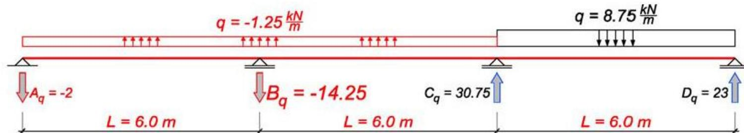
$$M_{1q} = -\left(\frac{-1.25}{15} + \frac{-1.25}{20} - \frac{8.75}{60}\right) \times 6.0^2 = 10.5 \text{ kNm} \Rightarrow A_q = \frac{-1.25 \times 6.0}{2} + \frac{10.5}{6.0} = -2.0 \text{ kN}$$
