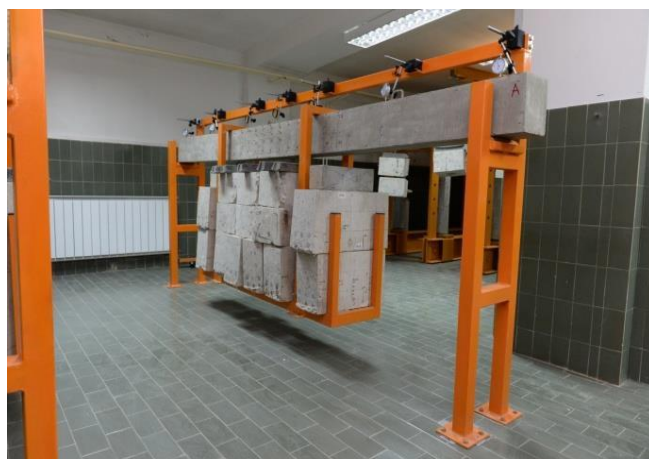
Testing the long-term behaviour of RAC beams (left and right)
