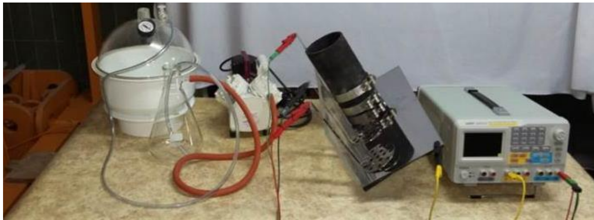
Chloride migration coefficient (NT492)—testing equipment
