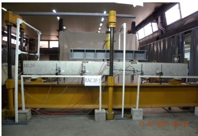
Testing of RAC beams in bending (left) and shear (right)
