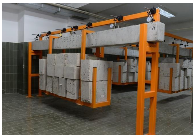
Testing the long-term behaviour of RAC beams (left and right)
