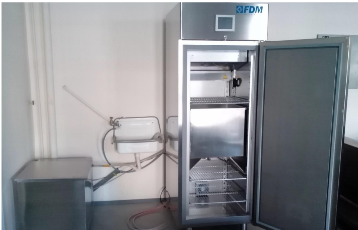
Climate chamber with a pool system for testing the freeze-thaw resistance of concrete
